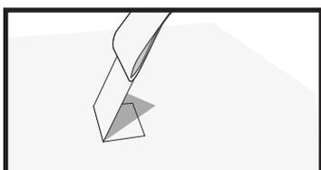
With a TESA® 7476 adhesive tape, or an equivalent, apply on an area of 2.5 cm x 5 cm (1 in x 2 in) plus some leftover space to allow for fingers to hold it. Fold and quickly pull off perpendicularly to the surface. No trace should remain on the removed adhesive. Repeat this operation in several places.
